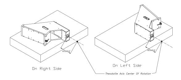
Figure 5 HUD Simulator views keeping the center line stationary.
