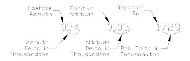
Figure 7. Example calibration numbers
