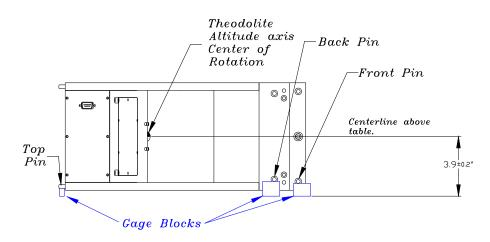
Figure 6. HUD Simulator in side position (View from back)
